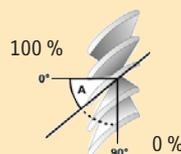
With this parameter the intermediate position 1 "slats" is defined. The set value in % refers to the parametered complete slats turn of the corresponding blind of the menu index card Motor 1 ... 4/Motor 1 - 4.
