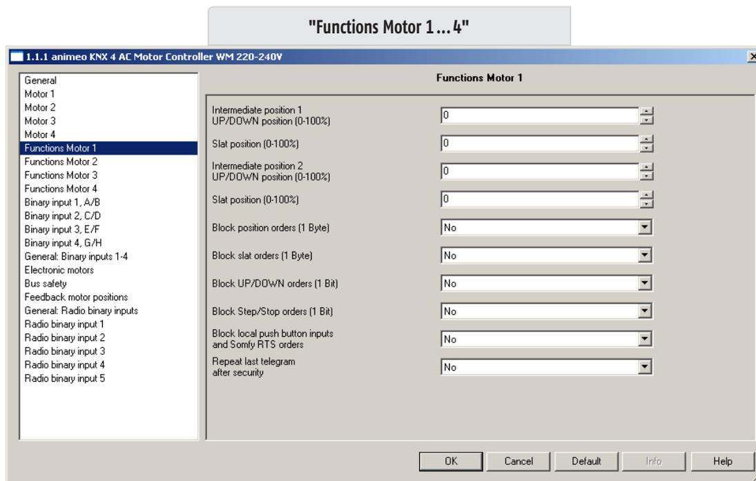
Four single menu index cards (Functions motor 1 ... 4) become visible if on the menu card index "General", the basic setting of the blinds on "Individual" is parametered. A menu index card (Motor 1 - 4) becomes visible if on the menu card index "General", the basic setting of the motors is parametered to "Combined".
