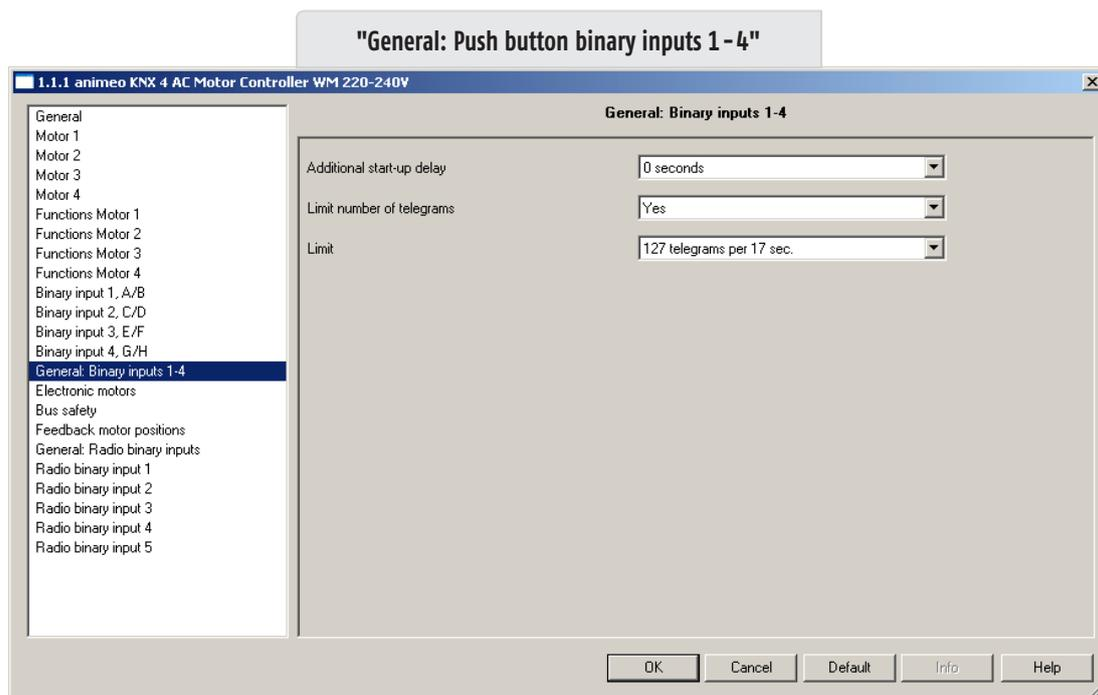
The parameters set here refer to the push button inputs 1 - 4.
