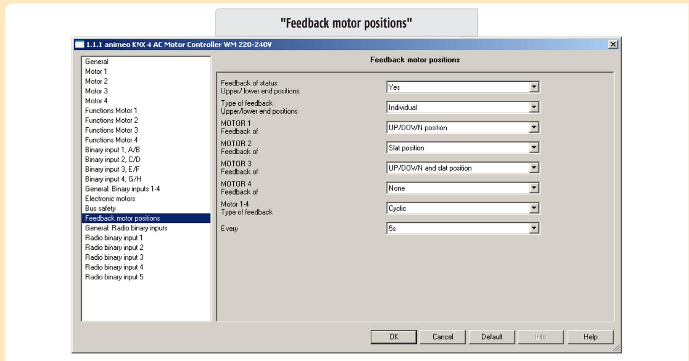
On this menu index card the parameters can be selected to announce the position status of the individual blinds on the bus. In addition, the generated status positions are based on the parametered move times and turn times of the menu index cards motor 1 ... 4 or motor 1 - 4.
