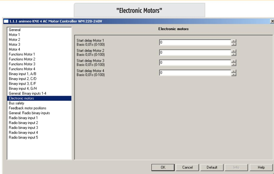
On this menu index card a start-up delay can be set for every single motor output.
