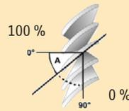
With this parameter the intermediate position 2 "Slats" is defined. The set value in % refers to the parametered complete slats turn of the corresponding Venetian blind of the menu index card Motor 1...4/Motor 1-4.
