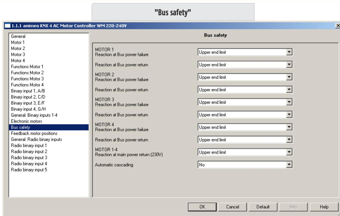
On this menu index card, the reaction can be defined for every single motor output with bus power failure and bus power return.
