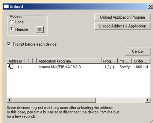
When the device has been programmed with the ETS software, a reset in the delivery state is no longer possible via the Rest/Prog button. Over the function "Unload" in the ETS, all settings of the device can be set back in the delivery state. The Reset/Prog button is then freed again.
