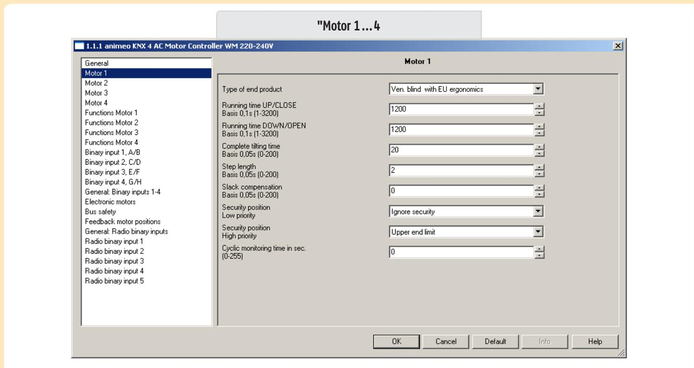
Four single menu index cards (motor 1 ... 4) become visible if in the menu of the basic setting "General" the parameter setting "Individual" is selected. One menu index card (motor 1 - 4) becomes visible if in the menu of the basic setting "General" the parameter setting "Combined" is selected.
